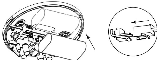
9. Mount luminaire housing on the base. Pay attention to the placement of lock latches. A "click" sound appears when closing the luminaire.
