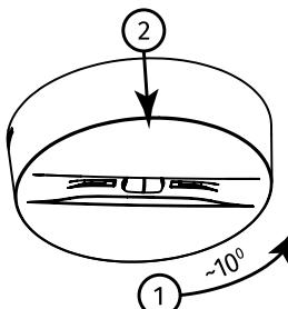
If there is a need to open a not mounted luminaire, use a small flat screwdriver, insert it from top next to the latch (ceiling facing side from luminaire base) and unbend the housing gently to release the latch from the catch.
