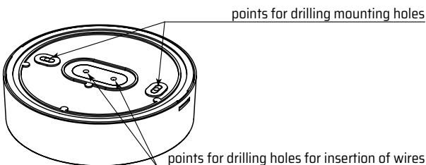
3. Drill holes in a ceiling according to mounting hole spacing (see DIMENSIONS) and in case of ROAD PLUS in the light direction (see OPTICS), so that the cables coming from the ceiling go freely through the hole provided for this purpose. Use Ø6-Ø8mm dowels and Ø4mm screws, suitable for surface material to which the luminaire is mounted.
