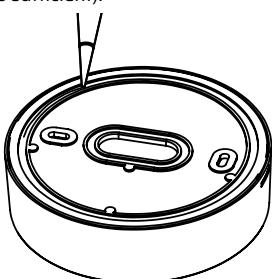
5. Insert the power cable and the communication cable (for CT) through the hole in the luminaire base and screw it to the ceiling.
